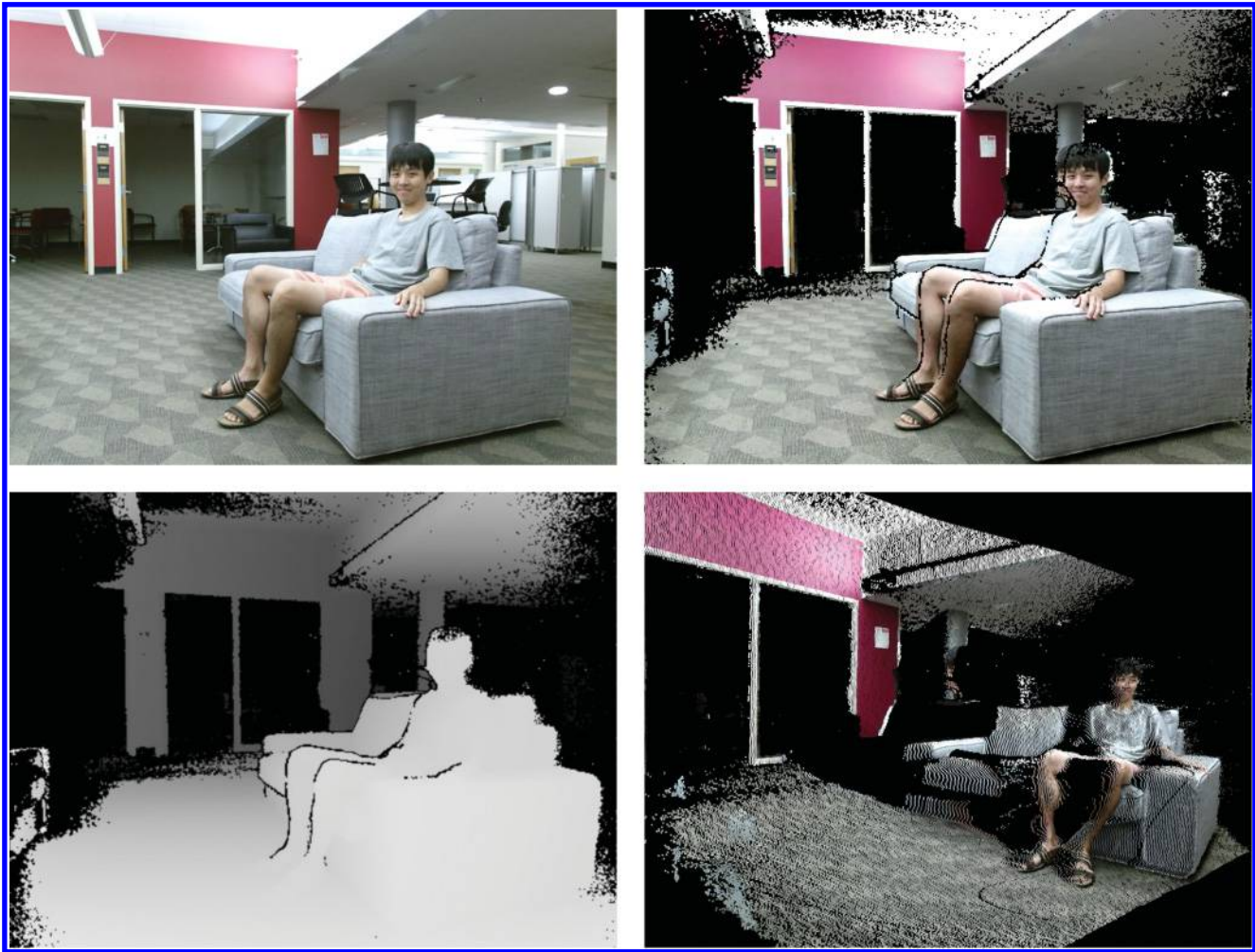
Figure 2. An example of our rendering technique. The top-left and the bottom-left are the color and depth pixels from a Kinect v2. The top-right is the rendered scene captured from a front-view, and the bottom-right is the rendered scene captured from a side-view.
