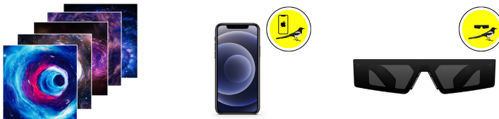
Fig. 2. Social Wormholes comprises three components (left to right): a set of printed markers which serve as endpoints for connections, a setup app for establishing connections between endpoints, and a connection app to receive and transmit content. Each person in a pair must have access to all components to use the system.
