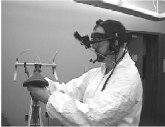
Worker in field wears head-mounted camera, microphone, and speaker
