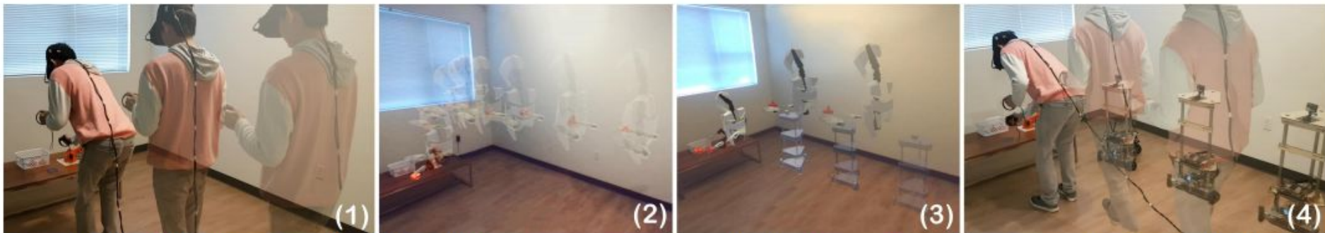
Figure 1: GhostAR workflow. To author HRC tasks that achieve time-space coordination, (1) user first authors a human ghost by recording his body movement, (2) then using the ghost as a visual reference, (3) author collaborative robot actions. (4) When acting the task, our system's collaborative model captures the body movement as input, maps it with the authored human motion, and outputs the corresponding collaborative robot motion.
